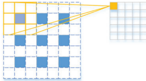
Figure 8: Schematic diagram of deconvolution
