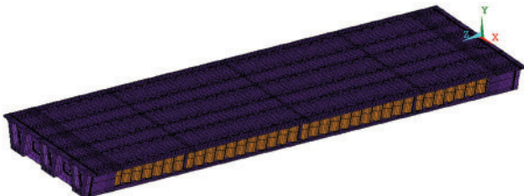
Figure 12: Finite element model of the bridge
