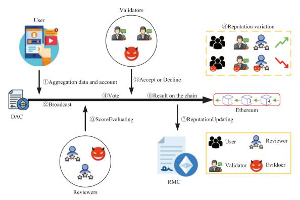
Figure 8: The workflow between application and contract layers
