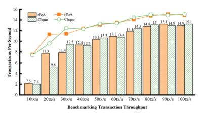
Figure 9: Transaction throughput comparison between rPoA and clique
