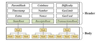
Figure 5: Block structure of Ethereum
