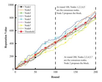
Figure 11: The variation of reputation values with reference to the reputation thresholds in DRM
