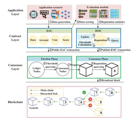
Figure 1: Layered structure of the proposed DRM mechanism and workflow
