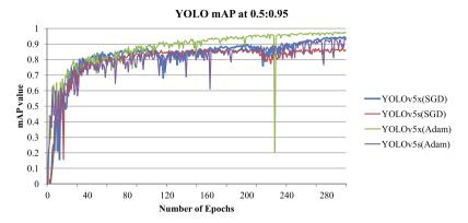
Figure 9: Mean Average Precision (mAP) at 0.5:0.95 for different YOLOv5 models
