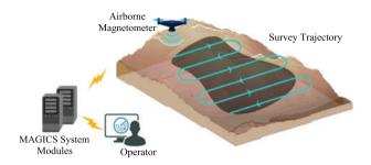
Figure 2: The default scenario of MAGICS, which plans the mission, classifies and localizes the landmines and reports on results
