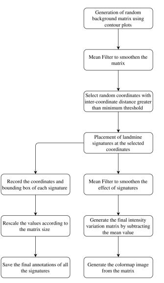
Figure 7: Steps involved in the generation of simulated Magnetometry colormap image
