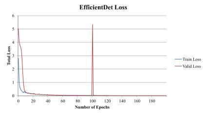
Figure 12: Total training and validation loss for EfficientDet-D0
