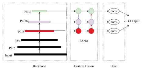
Figure 4: General architecture of YOLOv5
