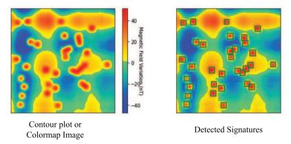
Figure 8: Magnetometry image sample from the simulated dataset and the detection results
