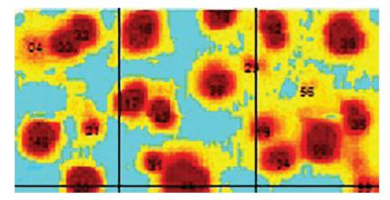
**Figure 6:** Cropped section of a magnetic map from a surveyed region using the MagDroneR4 UAV-Magnetometer [42]
