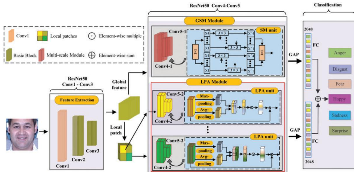
**Figure 2:** The structure of the GSM-LPA network. It contains four main parts, i.e., a feature extraction module, a global multiple-scale module (GMS), a local patches attention module (LPA), and a model-level fusion model. GAP presents a global average pooling operation, and FC presents a fully connected operation
