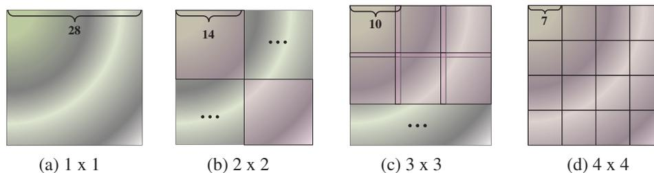
**Figure 8:** Four kinds of deep feature map segmentation strategy. (a) treats whole feature maps as an input feature map, which can be represented by one  $1 \times 1$  vector. (b) divides the whole feature maps into four patches, which can be represented by one  $2 \times 2$  vector. (c) divides the whole feature maps into nine patches, which can be depicted by one  $3 \times 3$  vector. (d) divides the whole feature maps into 16 patches, which can be represented by one  $4 \times 4$  vector
