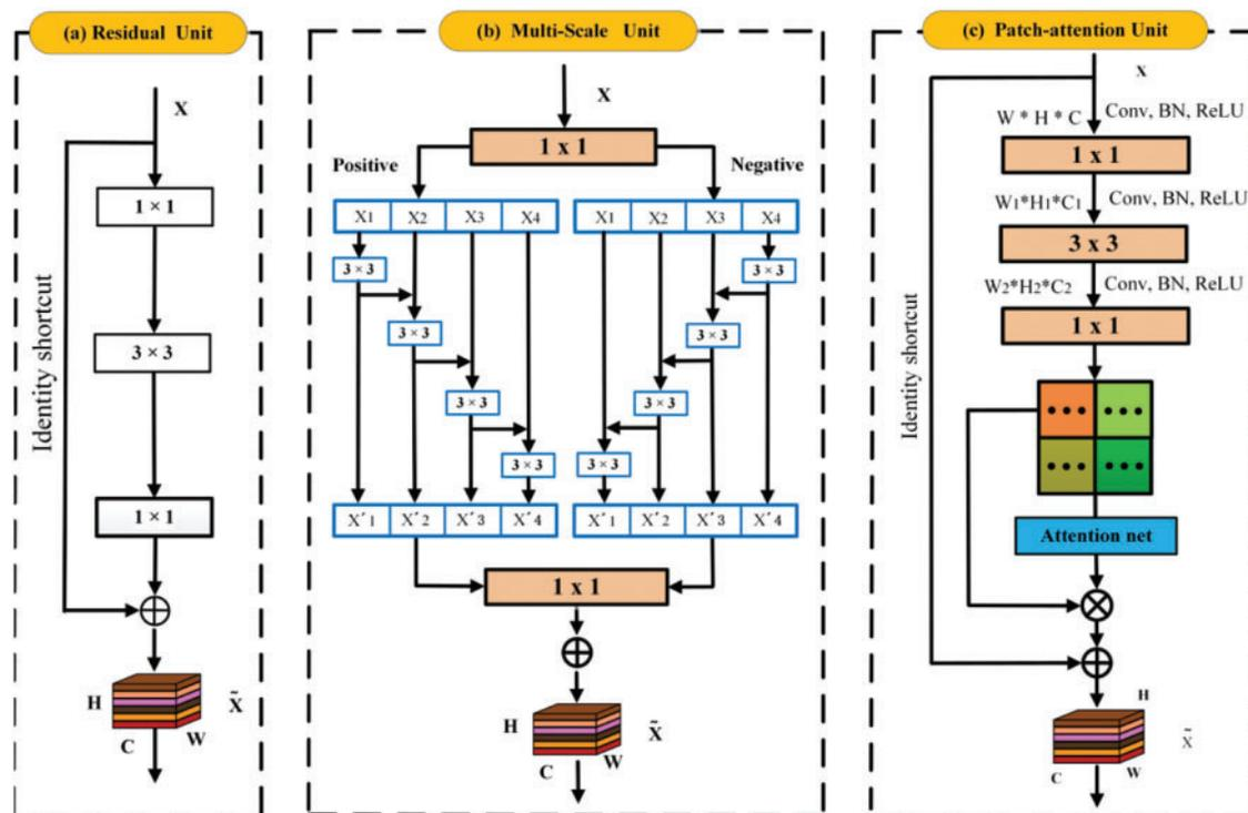
**Figure 3:** Three types of primary units are utilized in the GMS-LPA network, where (a) is the classic residual unit, (b) is the multiple-scale unit, and (c) is the local patches attention unit
