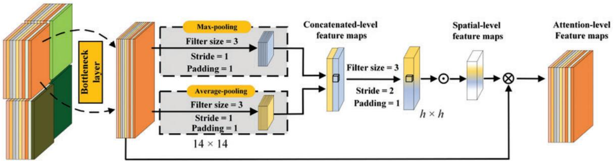
**Figure 5:** The structure of the local patch attention block.  $h$  is the size of feature maps after the concatenated-level convolution layer and  $\odot$  is a sigmoid function
