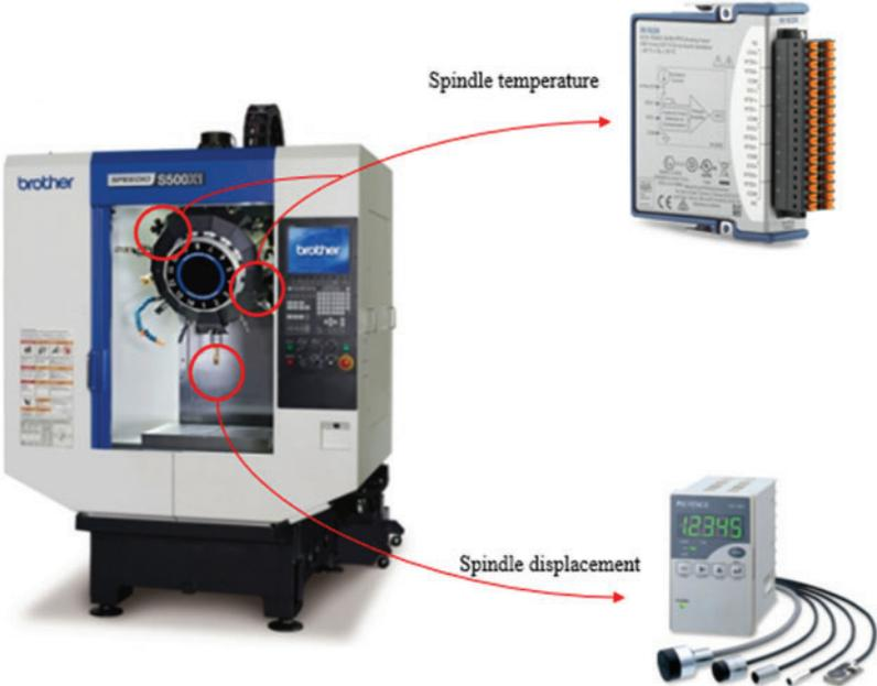
Figure 1: Layout of lab equipment
