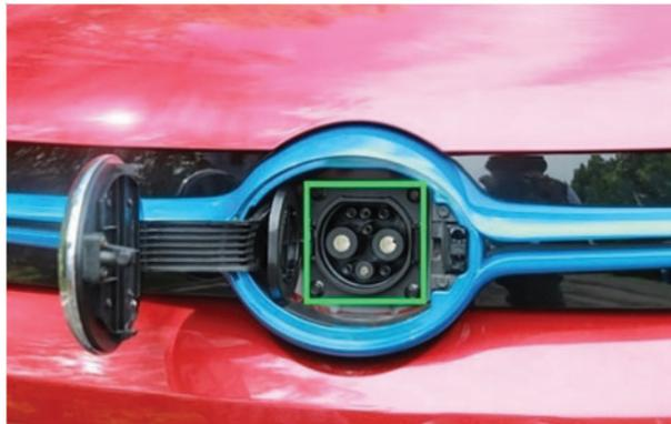
**Figure 4:** YOLO identification charging port
