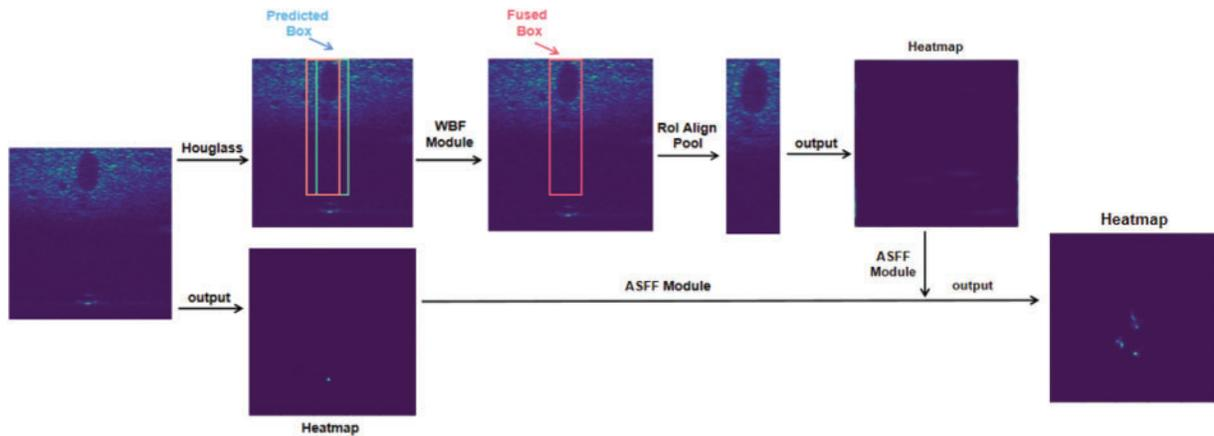
**Figure 2:** Acoustic shadow capture and fusion diagram
