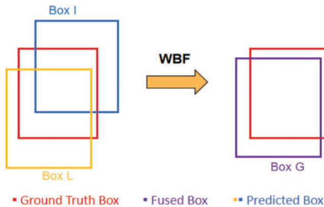
**Figure 3:** Weighted box fusion process
