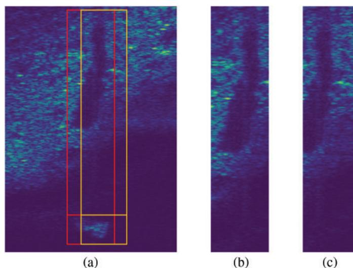
**Figure 8:** WBF module compared with the acoustic shadow box obtained from the reference model: (a) the red box is the acoustic shadow box obtained by the WBF module, and the yellow box is the acoustic shadow box obtained by the reference model; (b) acoustic shadows cut off by our model; (c) acoustic shadows from the final cut of the reference model
