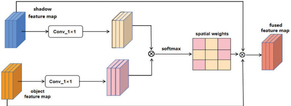
**Figure 4:** The structure of adaptive spatial feature fusion module. Acoustic shadow feature map captured and target object feature map are passed through  $1 \times 1$  convolution is adjusted to the same size. Concat and Softmax function are used to generate spatial feature fusion weights. Finally, two feature maps are multiplied and added to generate fusion feature maps
