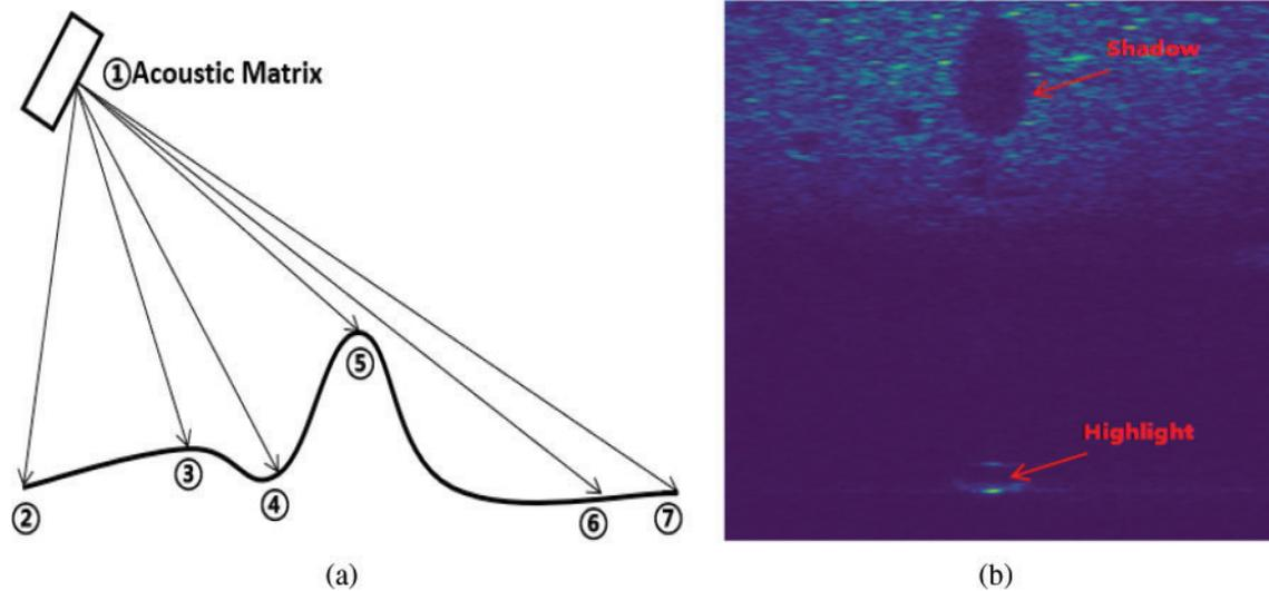
**Figure 1:** Schematic diagram of forward looking sonar imaging principle: (a) emits acoustic signals; (b) highlights and shadows in sonar images
