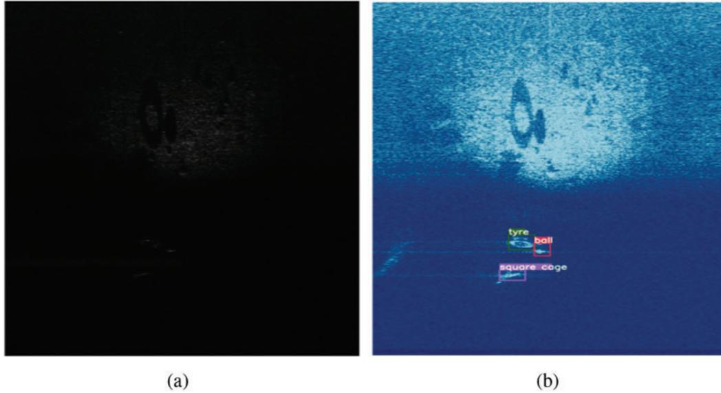
**Figure 7:** Sonar image data collection example: (a) original sonar image without gain adjustment; (b) after histogram equalization of (a)
