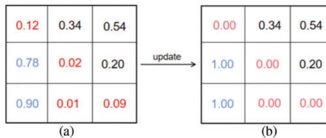
**Figure 6:** Threshold processing module example: (a) the fusion weights generated by ASFF; (b) the fusion weight after threshold module processing
