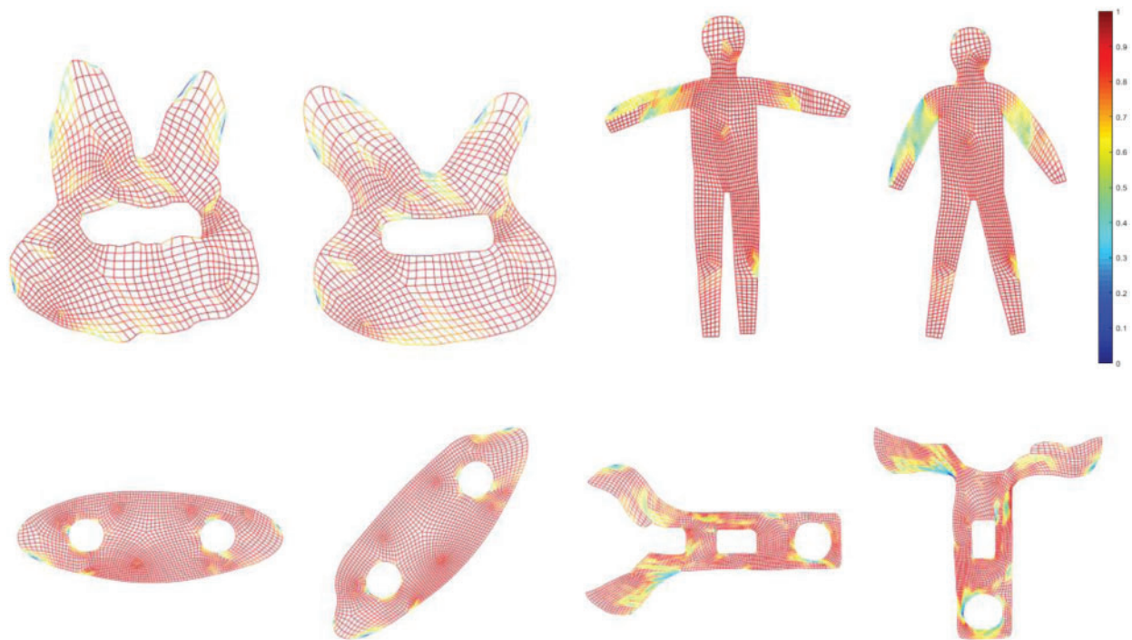
Figure 9: Colormap of the scaled Jacobian matrix on the iso-parametric edges in the source and target models whose parameterization was obtained by transfer. The first and third columns show the colormaps of the source model, and the second and fourth columns show the colormaps of the target model
