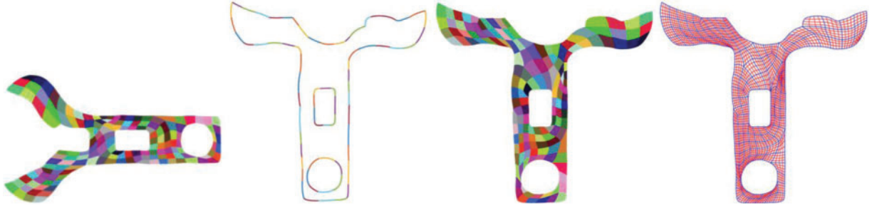
Figure 8: Results for different models by parametrization transfer. The left-most figure shows different source models. The second column of the above figure shows the target model. The third column shows the result obtained by our algorithm that transfers the source model to the target model. The rightmost figure above shows the iso-parametric lines of the resulting surfaces
