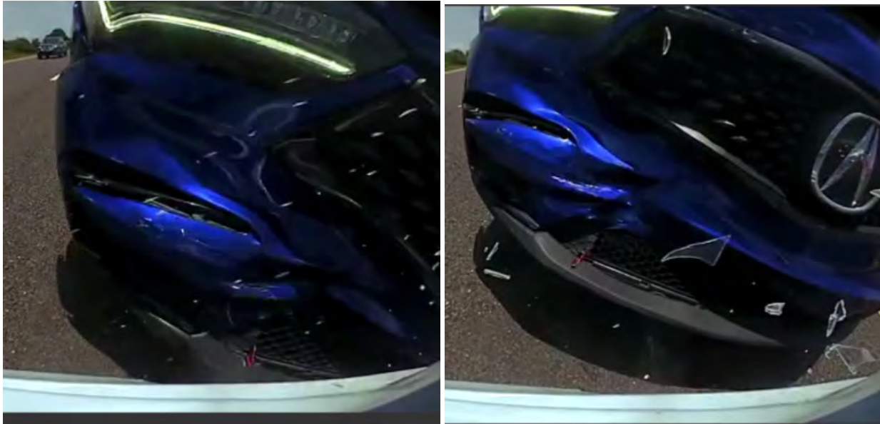
Figure 145: Tesla crash (Section 14.1). July 2020. The fast-coming blue car rear-ended the Tesla, indented its own front bumper, with flying broken glass (or clear plastic) cover shards captured by the Tesla rear camera [382]. See also Figures 143, 144, 146. (Data and video provided by QuantivRisk.)
