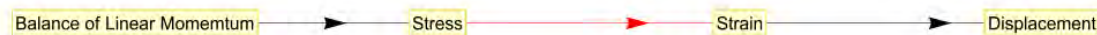
Figure 105: Single-physics block diagram (Section 11.2). Single physics is an easiest way to see the role of deep learning in modeling complex nonlinear constitutive behavior (stress-strain relation, red arrow), as first realized in [23], where balance of linear momentum and strain-displacement relation are definitions or accepted “universal principles” (black arrows) [25]. (Figure reproduced with permission of the authors.)
