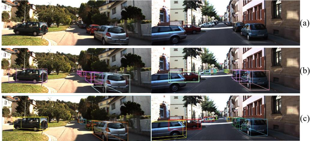
**Figure 5:** Comparative performance of MV3D and our method on 3D box generation. (a) The original images; (b)MV3D; (c) The proposed method. Notice that MV3D manages small vehicles well since the application of point cloud information. Although the proposed network slightly inferior to MV3D is small object, it achieves higher precision of bounding box location
