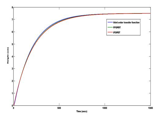
**Figure 5:** Comparison of time domain response of third order process with approximated IFOPDT and FFOPDT model
