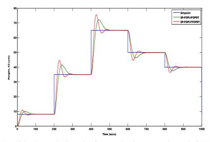
Figure 18: Height changes in the tank 3 for set point change at an interval of 200 seconds
