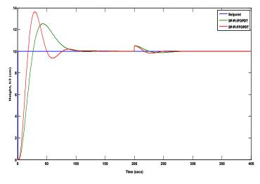
Figure 13: Closed loop response of smith based PI for integer model and fractional model with disturbance rejection
