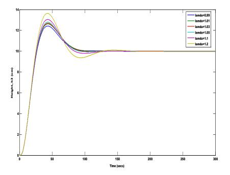
Figure 16: Effect of the closed loop response for FFOPDT process transfer function for varying value of lamda with fixed  $K_p$  and  $K_i$
