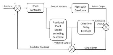
Figure 10: Smith predictor based FOPI with fractional model
