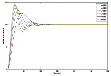
Figure 11: Effect of the closed loop response for varying value of  $\omega$  (Integer model)
