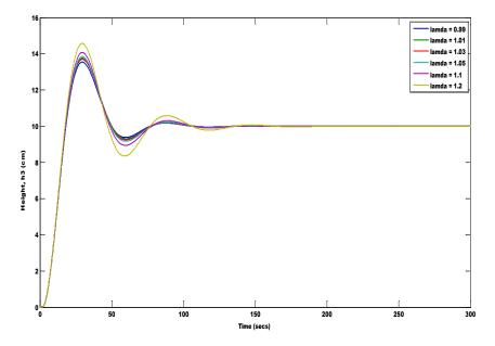
Figure 15: Effect of the closed loop response for IFOPDT process transfer function for varying value of lamda with fixed  $K_p$  and  $K_i$
