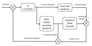
Figure 7: Smith predictor based PI with integer model
