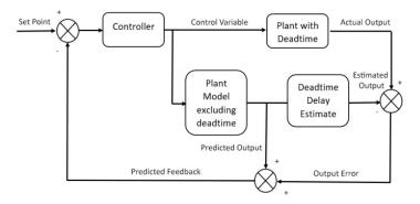
Figure 6: Structure of smith predictor controller
