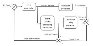
Figure 9: Smith predictor based FOPI with integer model
