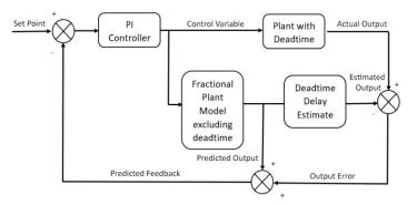
Figure 8: Smith predictor based PI with fractional model
