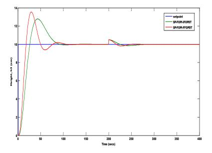
Figure 17: Closed loop response of smith based FOPI for integer model and fractional model with disturbance rejection
