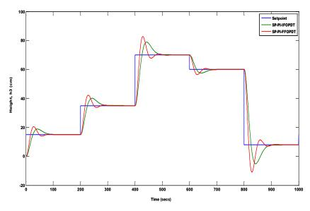
Figure 14: Height changes in the tank 3 for set point change at an interval of 200 seconds
