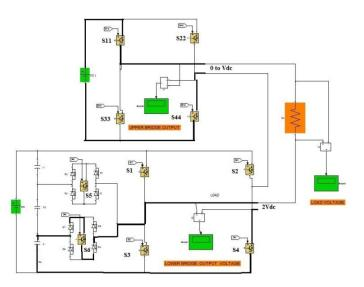
Figure e: Mode 5 operation of the proposed inverter
