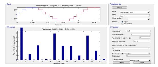
Figure 17: THD analysis of seven level inverter
