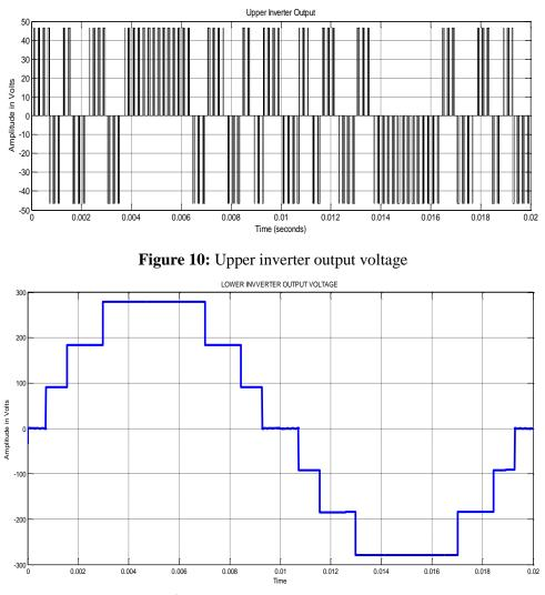
Figure 11: Lower inverter output voltage
