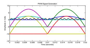
Figure 4: PWM signal generation of lower inverter
