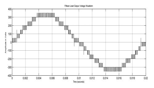
Figure 12: Fifteen level inverter output voltage
