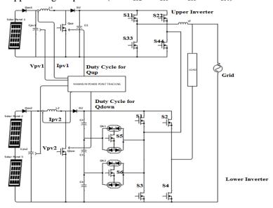
Figure 6: Schematic diagram of grid connected PV system
