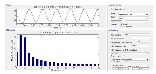
Figure 16: THD analysis of three level inverter
