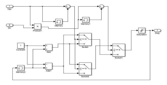
3.2 Simulink model of Perturb and Observe (P&O) MPPT algorithm
