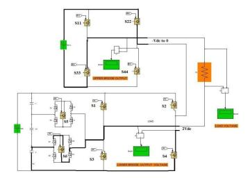
Figure f: Mode 6 operation of the proposed inverter
