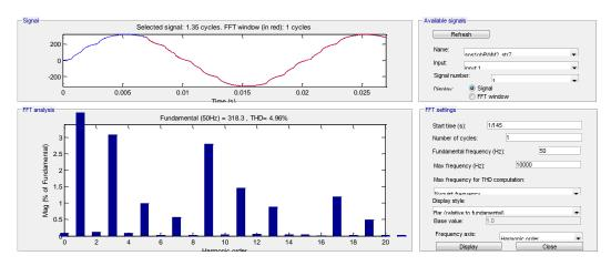
Figure 18: THD analysis of grid connected fifteen level inverter
