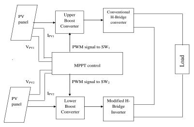
Figure 1: Block diagram of the proposed inverter
