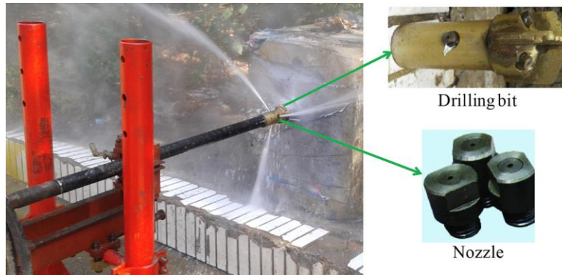
Figure 1: High-pressure water jet slotting technology
