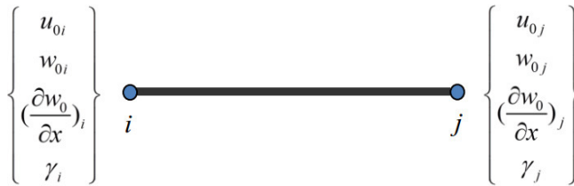
Figure 2: The nodal variables of the present two-noded element of shear flexible FG beams
