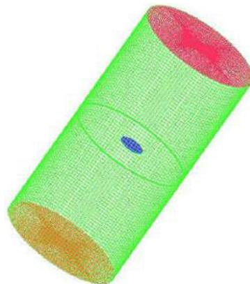
Figure 4: Structured quadrilateral for the far-field.
