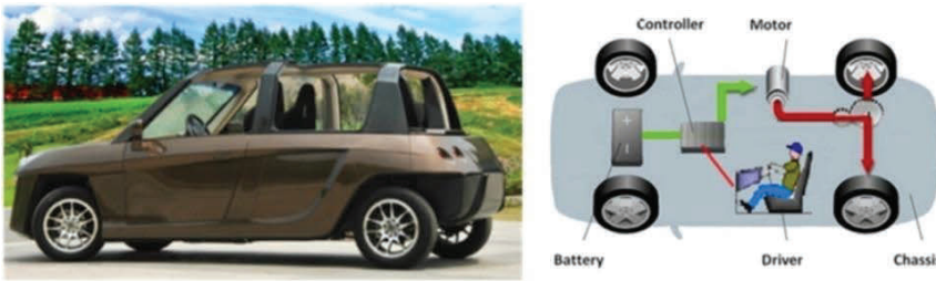
Figure 13: Pure electric vehicle: The appearance of the PEV (left) and the structure of the PEV (right)
