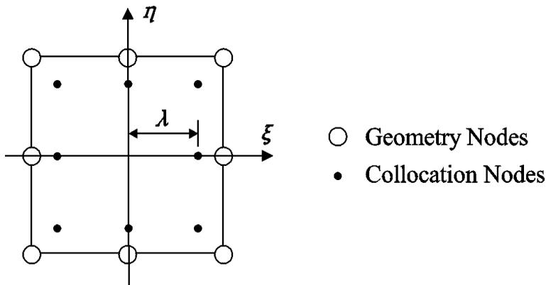
Figure 1: Eight-node discontinuous element
