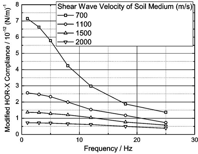
Figure 9:  $C_m$  at HOR-X direction
