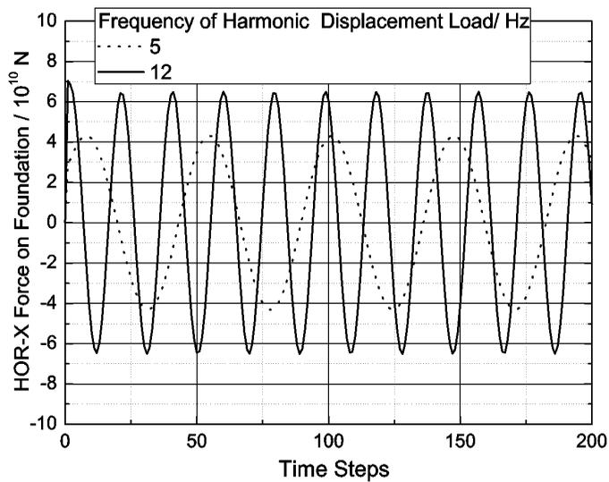
Figure 8: Horizontal reaction force of the foundation at  $f = 5.0$  and  $12.0$  Hz
