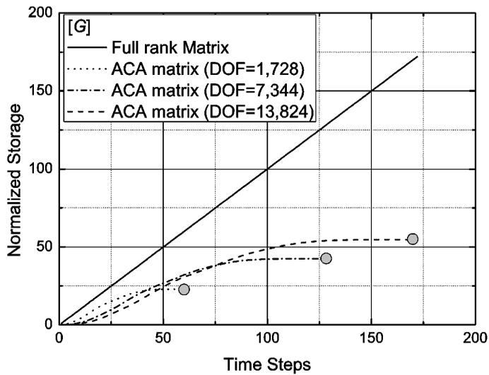
Figure 6: Storage of ACA-Compressed  $[G^n]$
