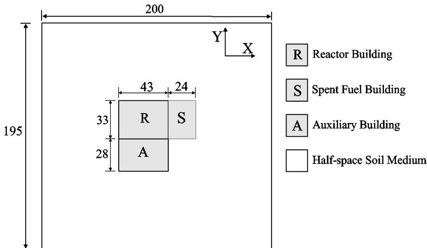
Figure 4: Sizes of the investigated domain containing HTR-PM nuclear island foundation and surrounding soil surface (unit: m)
