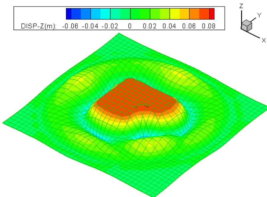
Figure 11: Vertical displacement at the 26-th time step ( $\text{DOF} = 7344$ ,  $f = 25.0$  Hz, No.2 soil properties)
