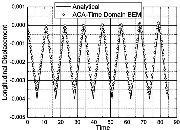
Figure 3: Longitudinal displacement at loaded end of the rod ( $\beta = 0.4$ )
