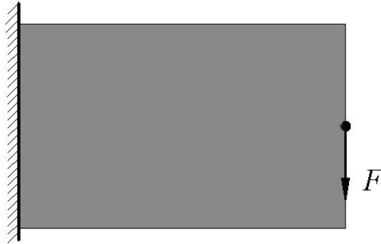
Figure 5: Design domain of a cantilever beam structure
