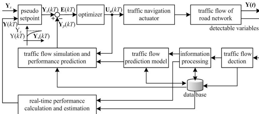
Figure 1: Architecture of traffic navigation predictive control system.
