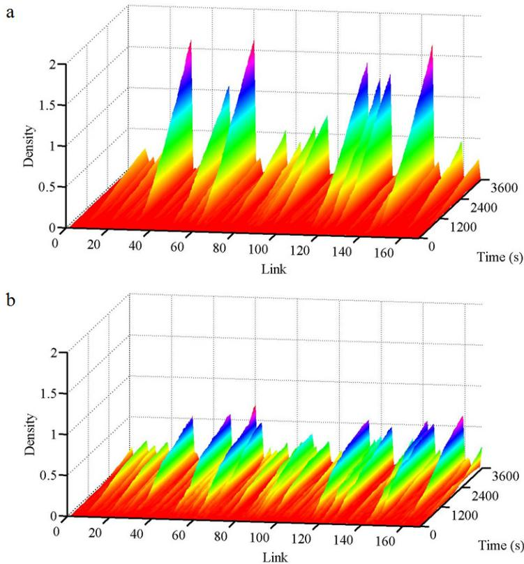
Figure 3: Link density. (a) is for static route guidance. (b) is for traffic navigation predictive control.
