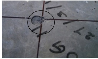
Figure 8: impression – 100 mm drop Figure 9: small crater – 200 mm drop
