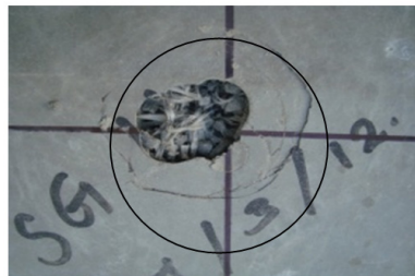
Figure 10: Protrusion of fibers on Figure 11: crater front side – 300 mm rear side - 300 mm drop
