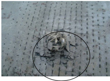
Figure 10: Protrusion of fibers on Figure 11: crater front side – 300 mm rear side - 300 mm drop
