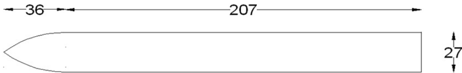
Figure 21: Projectile geometry (Dimensions in mm)
