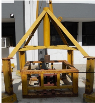
Figure 6: Drop weight testing frame
