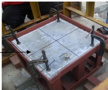
Figure 7: FABcrete panel with C clamps
