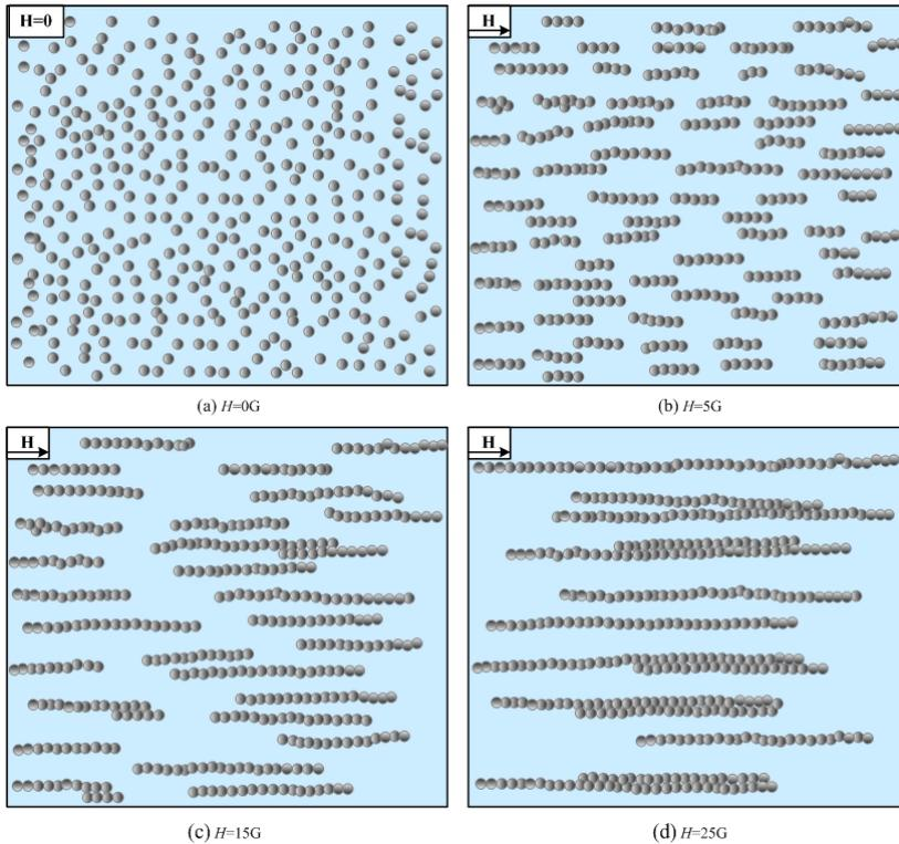
Figure 7: Influences of magnetic field strength on micro-structure in a two-dimensional area
