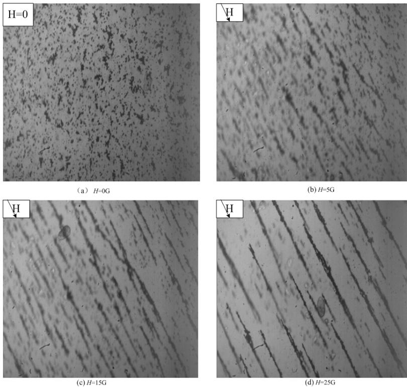
Figure 6: Video microscopy pictures of the micro-structure for different magnetic field strength
