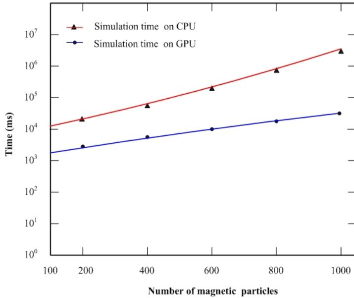
Figure 8: The simulation time of magnetic particles simulation system on GPU compared with on CPU
