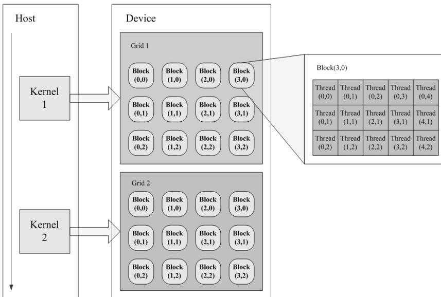
Figure 2: The GPU device architecture
