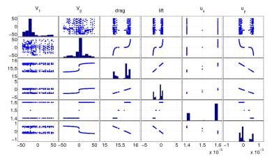
Figure 12: MOTS2 results on 4-objectives optimization scatter plot matrix. The order of lines and columns represents  $V_1$ ,  $V_2$ , drag, lift,  $u_x$ ,  $u_y$  respectively. Diagonal elements represent the corresponding histogram for each component.
