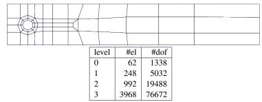
Figure 5: Coarse mesh with number of degrees of freedom for refined levels
