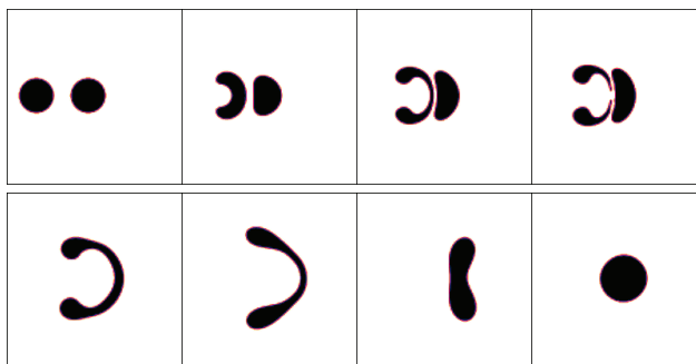
Figure 7: Case II, collision of two equally Droplets at different time steps for We=339 , Re=133.3 , X_c/D=1.5 , Laminar regime.
