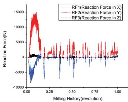
Figure 9: The reaction forces (MA=12°)
