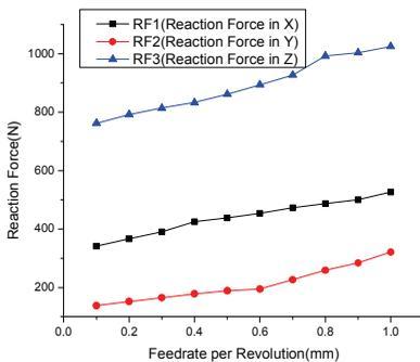
Figure 15: Reaction forces at various FPR
