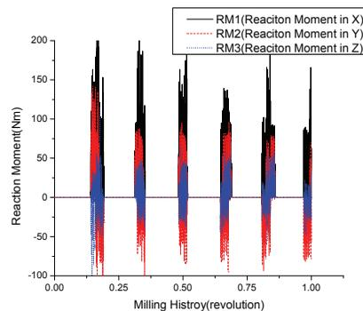
Figure 12: The reaction moments (FPR=0.9mm)
