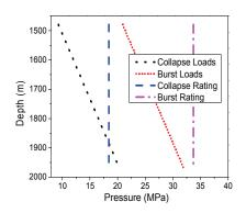
Figure 5: Casing strength check  $(40^\circ)$
