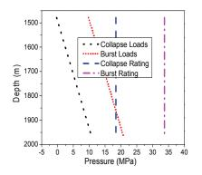
Figure 4: Casing strength check  $(30^\circ)$
