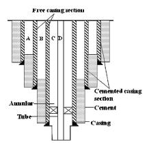
Figure 2: Schematic diagram of well structure
