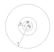
Figure 6: Casing-Cement-Formation System
