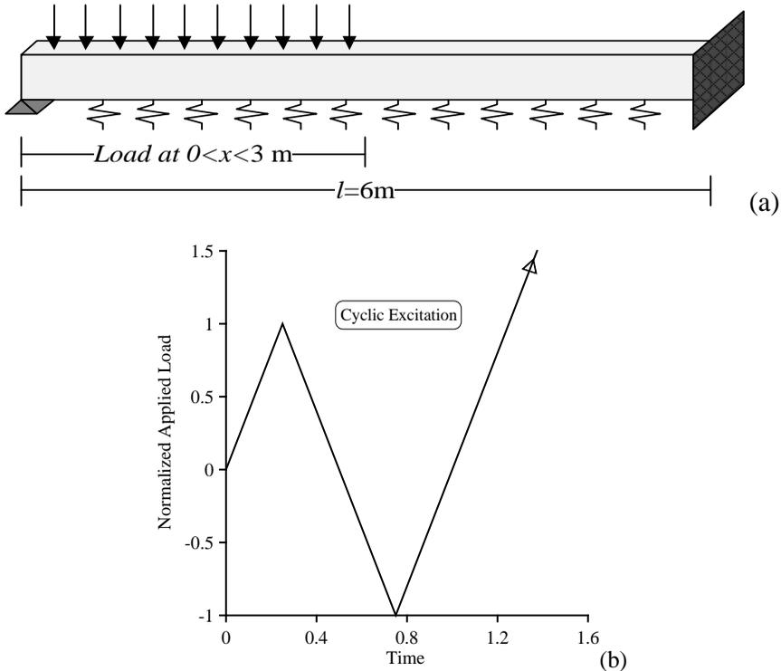
Figure 4: Pinned-fixed beam resting on an elastic-plastic Winkler foundation (a) subjected to a uniformly distributed cyclic loading (b).
