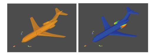
Figure 16: Finite element model of B727 (left) and its 9th eigenmode (right)
