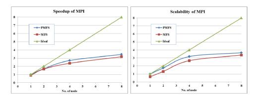
Figure 13: Parallel speedup and parallel scalability of PMFS and MFS with MPI
