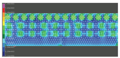
Figure 15: Normal stress distribution of the tensile direction ( $\sigma_{xx}$ ) of the specimen
