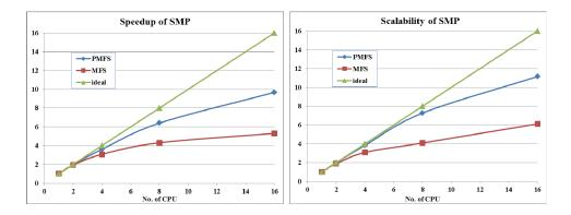
Figure 12: Parallel speedup and parallel scalability of PMFS and MFS in 16-way SMP
