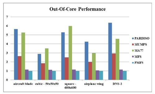
Figure 10: Elapsed time of the out-of-core solver performances scaled in terms of that of PMFS
