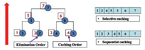
Figure 8: Data caching diagrams of the selective caching and sequential caching for a serial MFS
