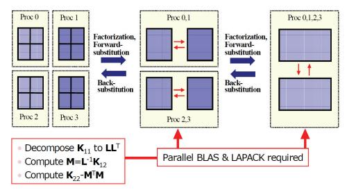
Figure 1: Parallel implementation of the distributed matrix factorization
