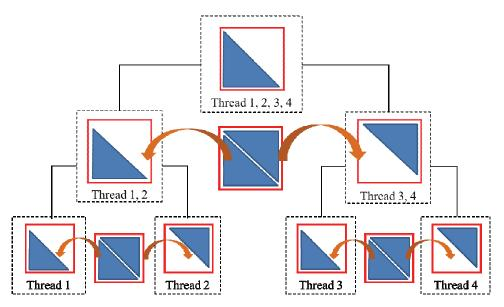
Figure 5: Basic concept of pairing two matrices for four threads case
