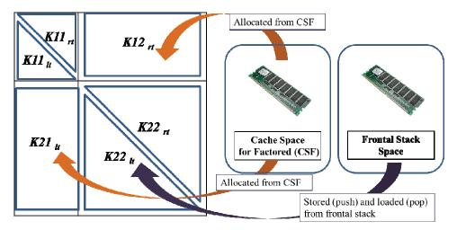
Figure 6: Splitting the Factorization Matrix - Triplet Factorization Matrix with pairing the sub-matrices
