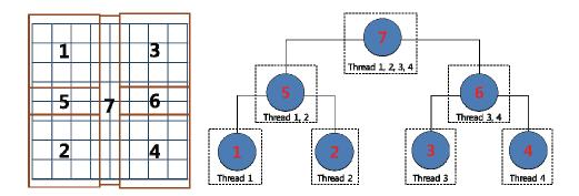
Figure 3: Finite element domain and its elimination tree of the four threads problem
