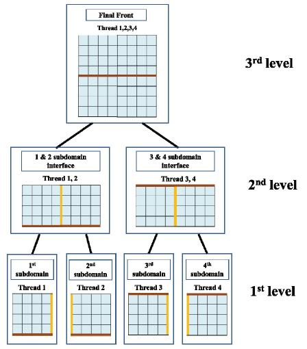
Figure 4: Elimination tree of multithreaded parallel factorization
