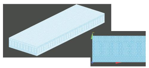
Figure 14: Finite element mesh of the specimen of the woven composite plate
