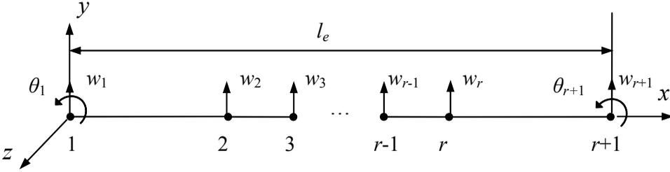
Figure 3: Layout of elemental nodes and the corresponding degree of freedom.
