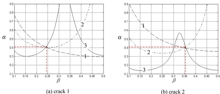
Figure 14: Frequency contours for case II ( $m = 30$ ) (1: The first order frequency contour; 2: The second order frequency contour; 3: The third order frequency contour)
