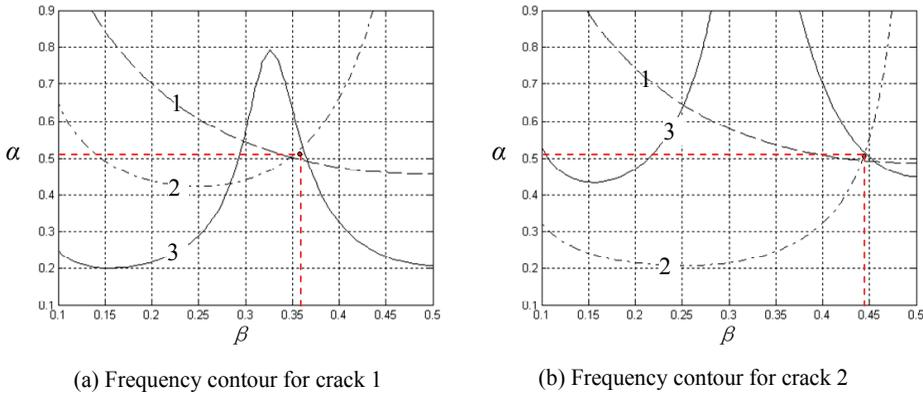
Figure 12: Frequency contours for case I ( $m = 10$ ) (1: The first order frequency contour; 2: The second order frequency contour; 3: The third order frequency contour)
