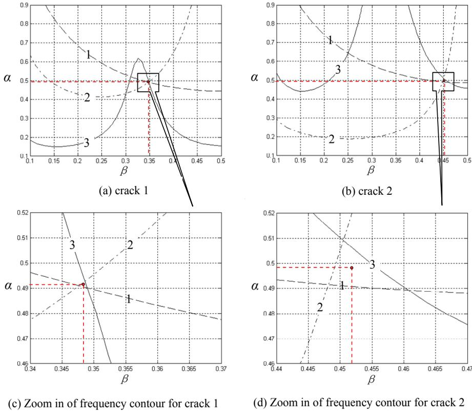
Figure 13: Frequency contours for case I ( $m = 30$ ) (1: The first order frequency contour; 2: The second order frequency contour; 3: The third order frequency contour)
