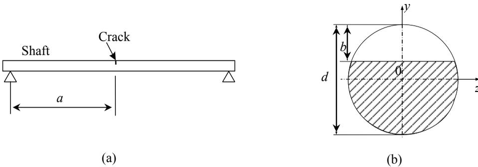
Figure 1: Crack parameters (a) Crack location (b) Crack depth.
