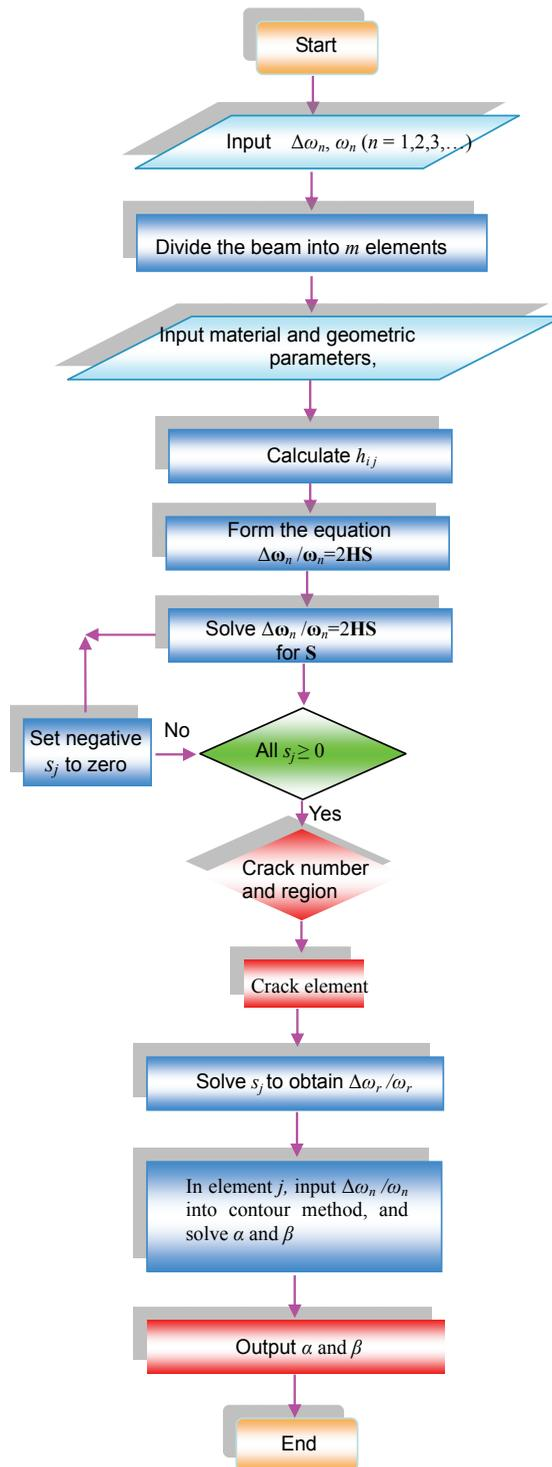
Figure 7: The block of algorithm for multiple cracks in rotor using WFEM
