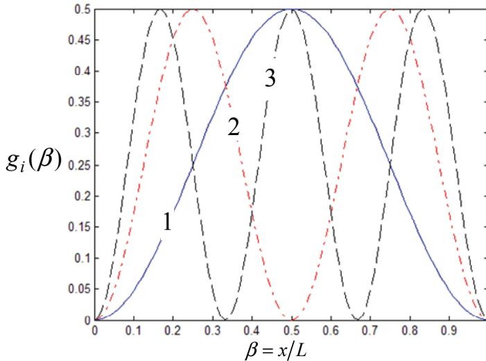
Figure 11: Simple supported rotor  $g_i(\beta)$  (1: The first order; 2: The second order; 3: The third order)
