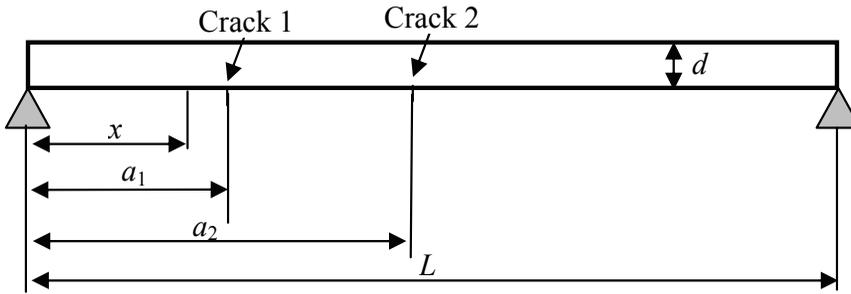
Figure 8: A rotor with two cracks
