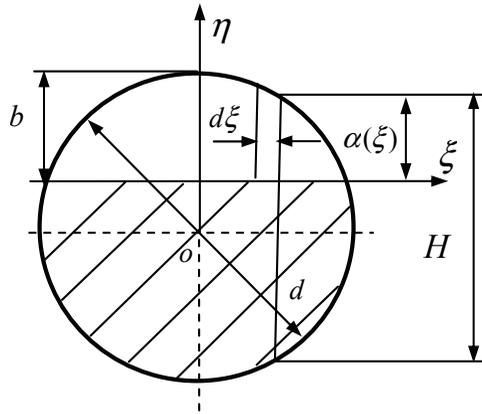
Figure 4: Geometry of a cracked section in rotor.
