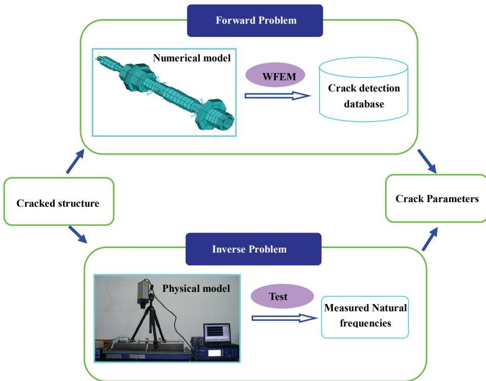
Figure 2: The process of crack identification
