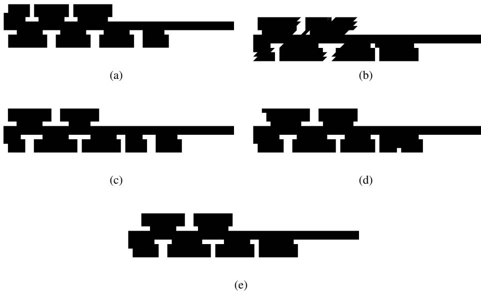
Figure 11: Our reanalysis topology optimization designs for : ( a) Q4-FEM, (b) T3-FEM, (c) CS-FEM ( nSD=2 ), (d) CS-FEM ( nSD=4 ), and (e) CS-FEM ( nSD=8 )
