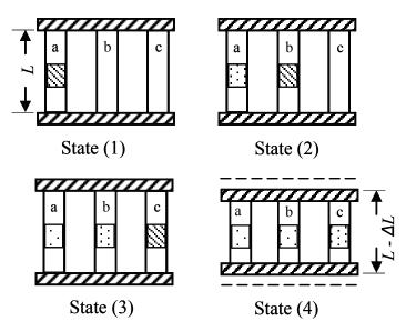
Figure 4: Mechanical model used to analyze the transverse component of inherent deformation
