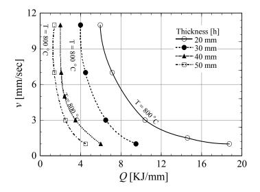
Figure 7: Relationship between neat heat input and speed of the heating source
