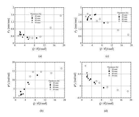
Figure 14: Relation between edge effect and heat input parameter  $Q/h^2$  at the exit plate edge (a) Longitudinal shrinkage, (b) Transverse shrinkage, (c) Longitudinal bending and (d) Transverse bending
