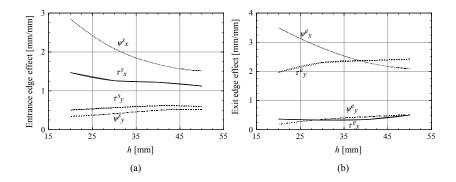
Figure 9: Variation of edge effect with plate thickness (a) entrance plate edge, (b) exit plate edge)
