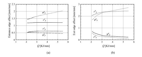
Figure 6: Variation of edge effect with heat input (a) entrance plate edge (b) exit plate edge
