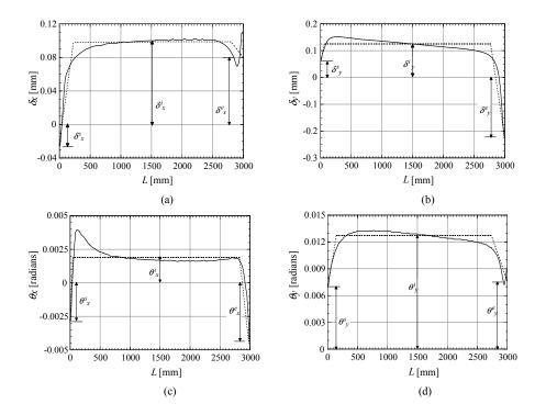
Figure 3: Comparison between computed and assumed distribution of inherent deformation (a) Longitudinal shrinkage, (b) Transverse shrinkage, (c) Longitudinal bending and (d) Transverse bending
