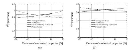
Figure 12: Variation of edge effect on transverse shrinkage with mechanical properties (a) entrance plate edge, (b) exit plate edge
