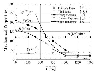
Figure 2: Mechanical properties of mild steel
