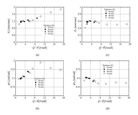
Figure 13: Relation between edge effect and heat input parameter  $Q/h^2$  at the entrance plate edge (a) Longitudinal shrinkage, (b) Transverse shrinkage, (c) Longitudinal bending and (d) Transverse bending
