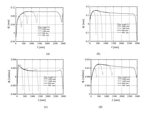
Figure 8: Variation of inherent deformation with plate length, (a) Longitudinal shrinkage, (b) Transverse shrinkage, (c) Longitudinal bending, and (d) Transverse bending
