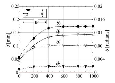
Figure 10: Variation of inherent deformation with the distance from the plate edge
