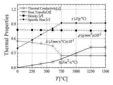
Figure 1: Thermal and physical properties of mild steel
