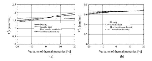
Figure 11: Variation of edge effect on transverse shrinkage with thermal properties (a) entrance plate edge, (b) exit plate edge
