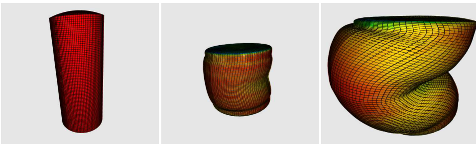
Figure 2: A cylinder, discretized in CUBIT, is compressed by rigid plates (not shown) until it buckles, introducing a large deformation.
