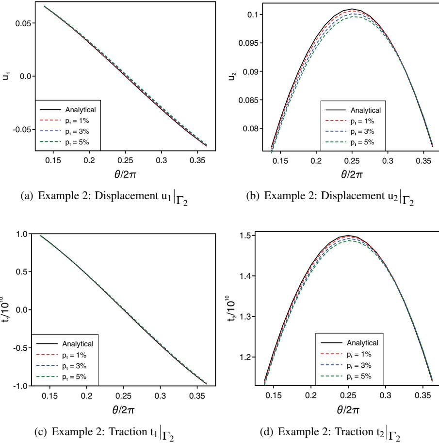
Figure 6: The analytical and numerical displacements (a)  $u_1|_{\Gamma_2}$  and (b)  $u_2|_{\Gamma_2}$ , and tractions (c)  $t_1|_{\Gamma_2}$  and (d)  $t_2|_{\Gamma_2}$ , obtained using the alternating iterative algorithm with initial guess  $\mathbf{u}^{(1)}|_{\Gamma_2} = \mathbf{0}$ , and various amounts of noise added into  $\mathbf{t}|_{\Gamma_1}$ , i.e.  $p_t \in \{1\%, 3\%, 5\%\}$ , for Example 2.
