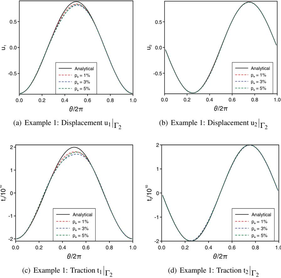
Figure 4: The analytical and numerical displacements (a)  $u_1|_{\Gamma_2}$  and (b)  $u_2|_{\Gamma_2}$ , and tractions (c)  $t_1|_{\Gamma_2}$  and (d)  $t_2|_{\Gamma_2}$ , obtained using the alternating iterative algorithm with initial guess  $\mathbf{t}^{(1)}|_{\Gamma_2} = \mathbf{0}$ , and various amounts of noise added into the displacement vector  $\mathbf{u}|_{\Gamma_1}$ , i.e.  $p_u \in \{1\%, 3\%, 5\%\}$ , for Example 1.
