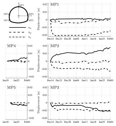
Figure 2: Histories of displacement components in x, y, and z directions measured at measurement points MP1 through MP5 of the *considered* measurement cross-section (MC1452)
