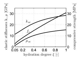
Figure 9: Evolution of elastic shear modulus  $\mu_{sc}$ , elastic bulk modulus  $k_{sc}$ , and uniaxial compressive strength  $f_c$  of shotcrete over hydration degree for w/c = 0.50 and a/c = 5, values predicted by the micromechanical models of [Scheiner and Hellmich (2009)], [Pichler, Hellmich, and Eberhardsteiner (2009)] and [Pichler, Scheiner, and Hellmich (2008)]
