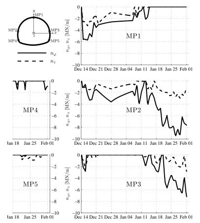
Figure 14: Evolution of circumferential and longitudinal normal forces acting at measurement points MP1 through MP5 of the *considered* measurement crosssection (MC1452) of the Sieberg tunnel
