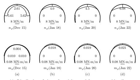
Figure 11: Distribution of circumferential normal forces  $n_{\varphi}$  and bending moment  $m_{\varphi}$ , at critical dates, for interpolation strategy I (a) Dec 15 (b) Jan 18 (c) Jan 20 and (d) Jan 22
