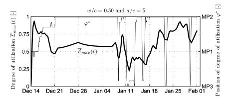
Figure 13: History of degree of utilization and its position for MC1452 of Sieberg tunnel using interpolation strategy II
