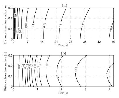
Figure 8: Evolution of hydration degree across the tunnel shell thickness: (a) from placement of shotcrete through 50 days, (b) zoom out for the first 4 days after placement of shotcrete
