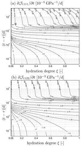
Figure 10: Creep rates of shotcrete with w/c = 0.50 and a/c = 5: (a)  $\partial \mathcal{J}_{1111}/\partial t$  and (b)  $\partial \mathcal{J}_{1122}/\partial t$ , values predicted by the model of [Scheiner and Hellmich (2009)]
