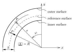
Figure 6: Definitions of reference surface and moving radial coordinate  $\rho$  of tunnel shell
