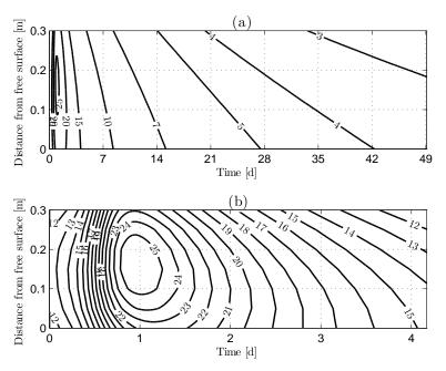
Figure 7: Evolution of temperature, across the tunnel shell thickness, due to heat of hydration: (a) from placement of shotcrete through 50 days (b) zoom out for the first 4 days after placement of shotcrete
