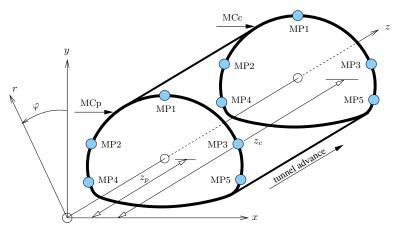
Figure 4: Illustration of the location, along *z*-axis, of the *considered* and *preceding* measurement cross-sections (MCc and MCp, respectively)
