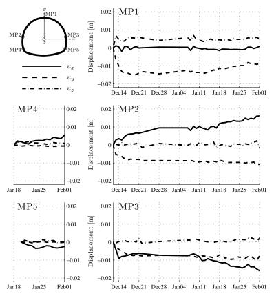
Figure 3: Histories of displacement components in x, y, and z directions measured at measurement points MP1 through MP5 of the *preceding* measurement cross-section (MC1444)
