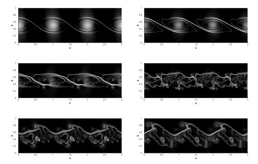
Figure 7: Development of a two-dimensional Kelvin-Helmholtz instability in the viscous and resistive MHD equations at  $Re = Sr = 10^5$  using a  $P_3P_5$  scheme. From top left to bottom right the density contours are shown at times t = 5, 6, 7, 8, 9, 10.
