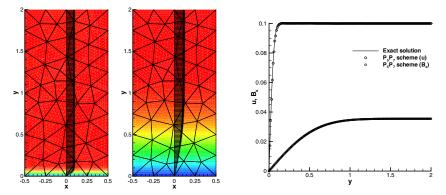
Figure 1: First problem of Stokes in 2D with a magnetic Prandtl number of  $Pr_m = 10^{-2}$ . Unstructured triangular mesh and distributions of velocity (left) and magnetic field (middle). Comparison of the numerical results obtained with a  $P_5P_7$  scheme and the exact solution at time t = 1 (right).
