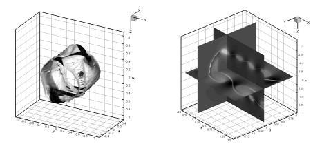
Figure 9: Viscous and resistive 3D Kelvin-Helmholtz instability according to Keppens and Tóth (1999) at t = 4.0 forcing the first mode (m = 1).  $Re = Sr = 10^4$ . Left: u = 0 iso-surface. Right: density contours in the cut planes x = 0, y = 0 and z = 0.
