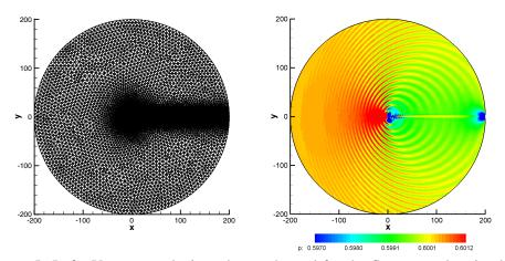
Figure 5: Left: Unstructured triangular mesh used for the flow around a circular cylinder at Re = Sr = 100. Right: Pressure contours in the far field at time t = 1000.
