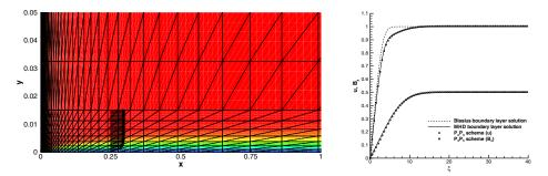
Figure 3: MHD boundary layer at  $Re = 10^6$  and  $Sr = 10^5$  over a flat plate. Unstructured triangular mesh,  $B_x$  contour colors and velocity vectors at x = 0.25 (left). Horizontal velocity and magnetic field profiles at x = 0.25 and comparison with the MHD boundary layer solution (right). For comparison purposes, also the standard Blasius solution at the same Reynolds number is indicated.
