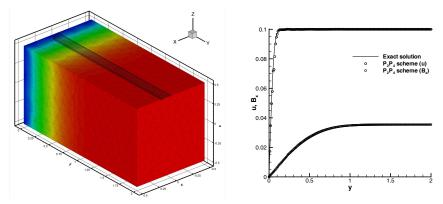
Figure 2: First problem of Stokes in 3D with a magnetic Prandtl number of  $Pr_m = 10^{-2}$ . Unstructured tetrahedral mesh and contour levels of the magnetic field component  $B_x$  (left). Comparison of the numerical results obtained with a  $P_2P_4$  scheme and the exact solution at time t = 1 (right).
