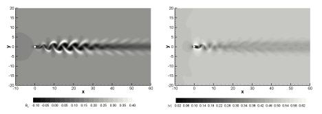
Figure 6: Left: Contour levels of the magnetic field component  $B_x$  in the cylinder wake at t = 1000. Right: Contour levels of the velocity magnitude  $|\vec{v}|$  in the cylinder wake at t = 1000.
