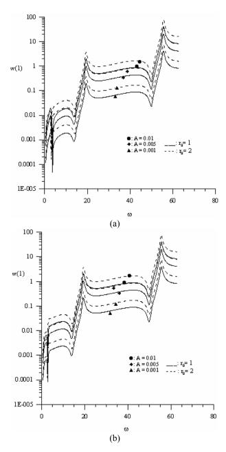
Figure 4: Influence of the excitation frequency  $\omega$ , the amplitude of excitation angle *A* and the root radius  $r_0$  on the tip amplitude of (a) an outward rotating beam and (b) an inward rotating beam. [ $m_{tip} = 0.1$ , C = 1].
