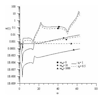
Figure 2: Influence of the excitation frequency  $\omega$ , the tip mass  $m_{tip}$  and the root radius  $r_0$  on the tip amplitude of an inward rotating beam.[A = 0.001, C = 1].
