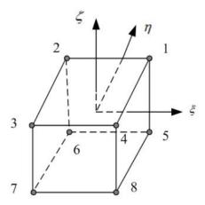
Figure 1: Solid element in referential coordinate system
