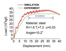
Figure 12: The load-stroke relation with R=1.6
