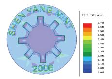
Figure 19: Effective strain contour of the first layer elements
