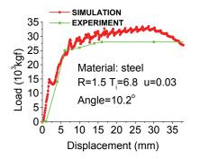
Figure 11: The load-stroke relation with R=1.5
