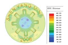
Figure 20: Effective stress contour of the first layer elements
