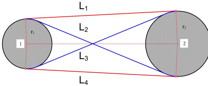
Figure 3: Hottel's method for two particles
