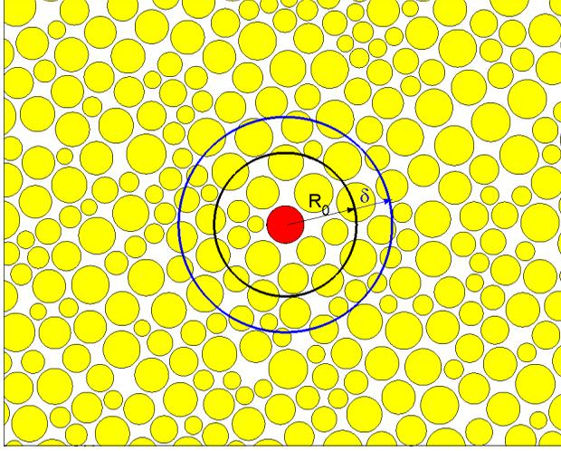
Figure 10: Definition of a circular cover domain and enlargement for a particle
