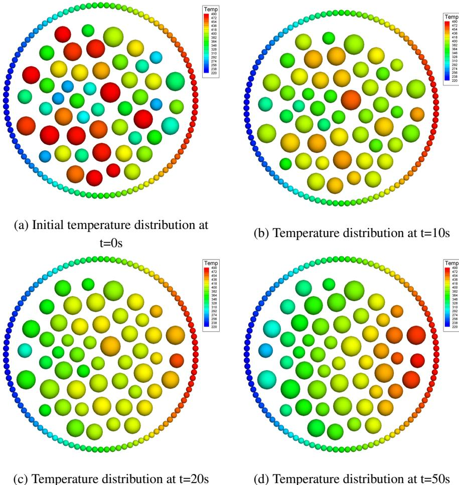
Figure 13: Temperature evolution of the particle assembly at several time instants
