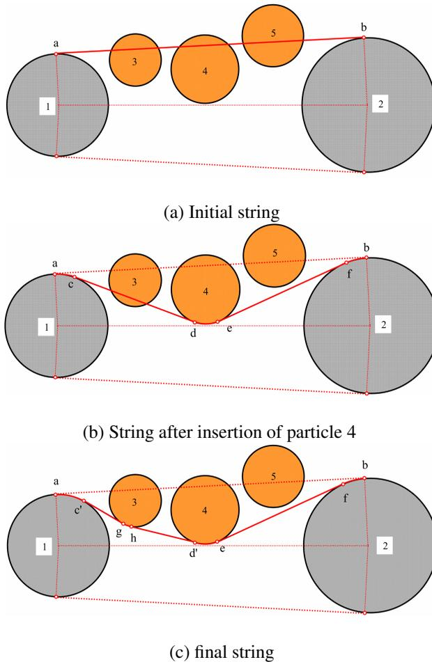
Figure 5: Generation of the upper uncrossed string between two particles with blockage
