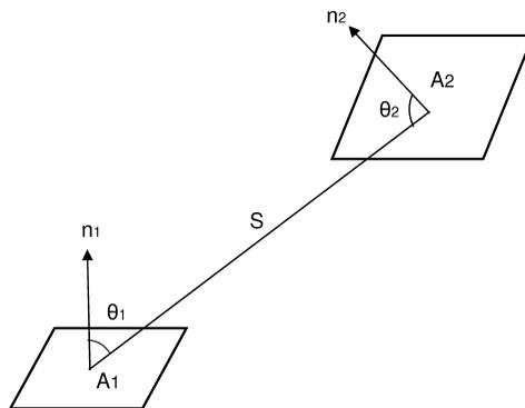
Figure 1: Geometric view factors between two finite surfaces
