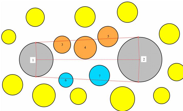
Figure 4: Two particles with blockage in a randomly packed bed of circular particles
