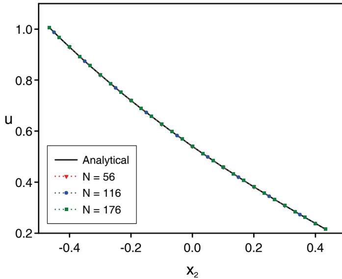
(a) Example 1: Temperatures on  $\Gamma_2$
