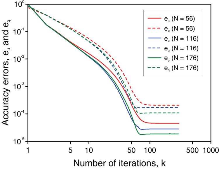
Figure 1: The accuracy errors,  $e_u$  and  $e_q$ , as functions of the number of iterations,  $k$ , obtained using exact Cauchy data on  $\Gamma_1$  and various numbers of MFS boundary collocation points, namely  $N \in \{56, 116, 176\}$ , for Example 1.
