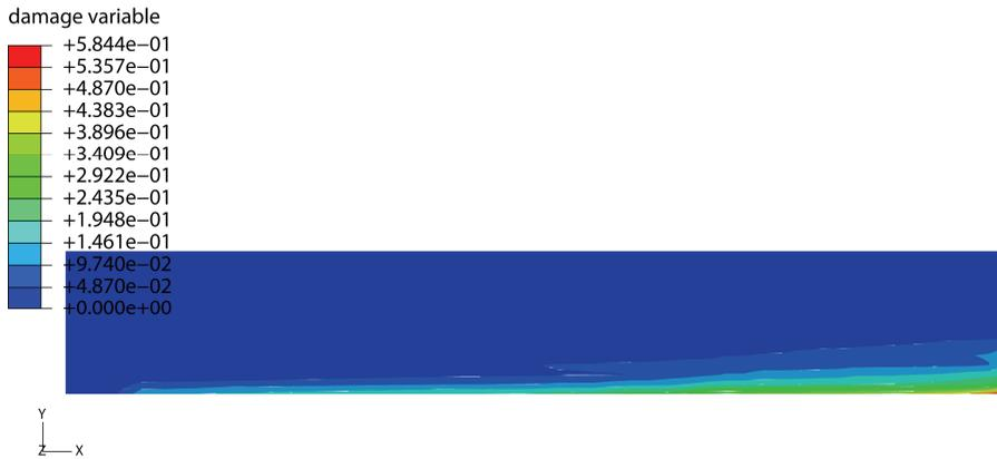
Figure 17: Damage distribution after 50 years of exposure
