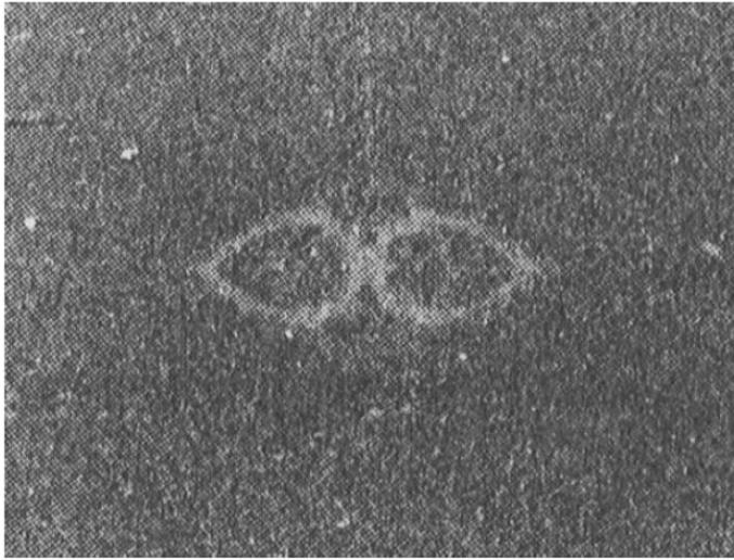
Figure 6: Experiment delamination in the plate [Choi and Chang (1992)]
