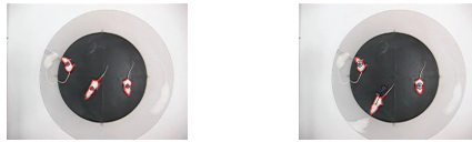
Figure 7: Tracking mice in a lab environment over 414 image frames: quick movement with severe direction changes can be correctly tracked by the proposed tracking framework.
