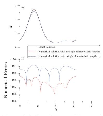
Figure 1: For a very slender ellipse with an aspect ratio 200, (a) comparison of the exact solution and numerical solutions obtained by a Single-Characteristic-Length Trefftz expansion and by a Multiple-Characteristic Length Trefftz expansion, and (b) comparison of the numerical errors.
