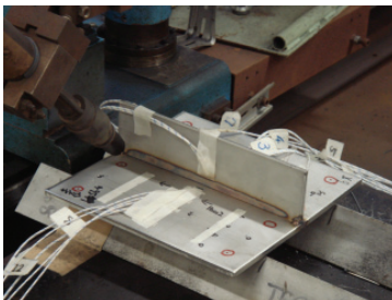
Figure 1: Experimental set-up of fillet welding
