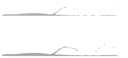
Figure 7: Jet configuration at t = 30 \mu\text{s} , MPM results on the top encounter numerical fracture and adaptive MPM results on the bottom avoid that problem. Particles that represent explosion products are removed for clarity.
