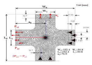
Figure 5: Specimen geometry
