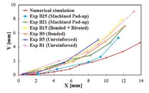
Figure 13: Predicted fracture path and experimental fracture paths
