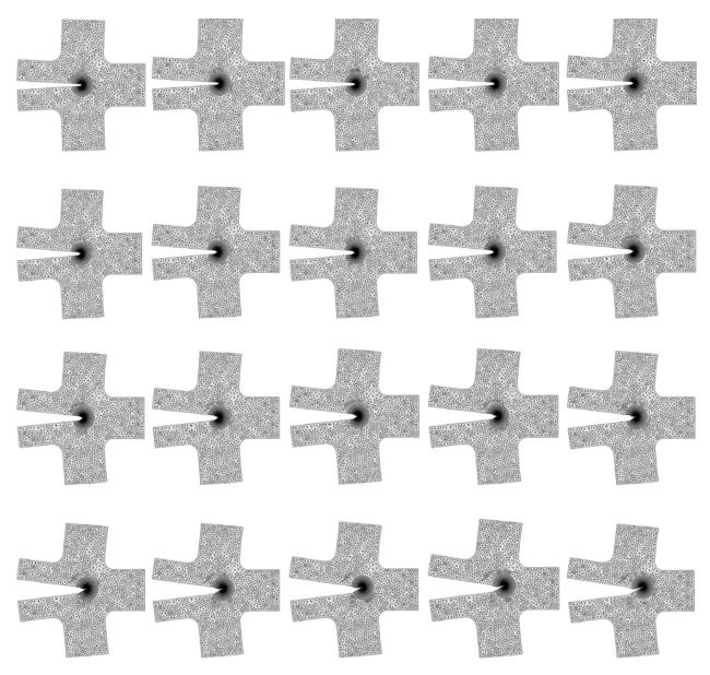
$0.79355 \le u_v$  [mm],  $3.00821 \le P_x$  [kN],  $0.0 \le a \le 14.7$  [mm] Figure 9: Mesh patterns on crack propagation progress
