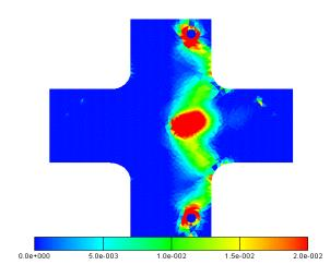
Figure 10: Equivalent plastic strain pattern
