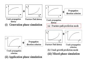
Figure 4: Types of fracture simulation
