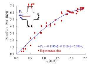
Figure 7: Relation between Displacement Uy and Shear Load Px
