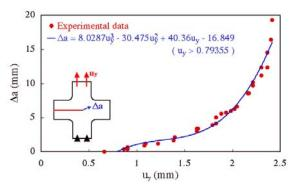
Figure 8: Relation between Displacement Uy and Crack Propagation Length  $\Delta a$
