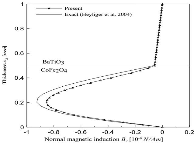
**Figure 13** : Through thickness distribution of the normal magnetic induction component  $B_2$ .
