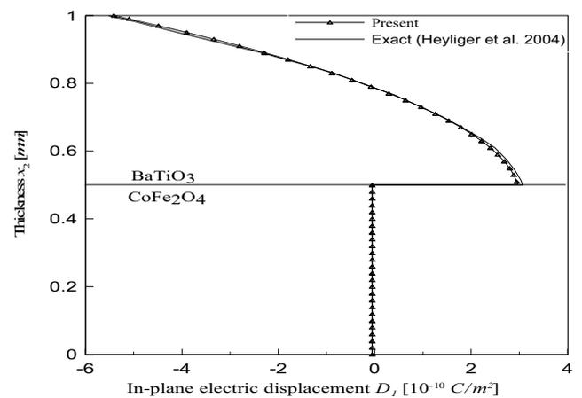
**Figure 10 :** Through thickness distribution of the in-plane electric displacement component  $D_1$ .
