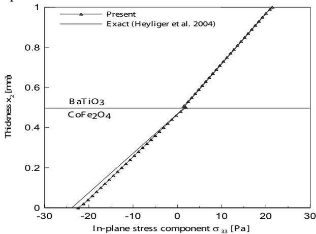
**Figure 7** : Through thickness distribution of the in plane normal stress  $\sigma_{33}$ .
