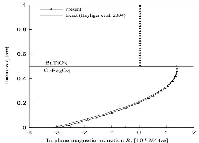
Figure 12 : Through thickness distribution of the in-plane magnetic induction component  $B_1$ .
