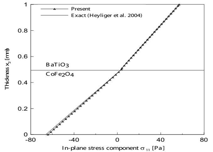
**Figure 6** : Through thickness distribution of the in plane normal stress  $\sigma_{11}$ .
