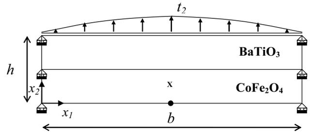
Figure 4 : Magneto-electro-elastic laminate scheme.
