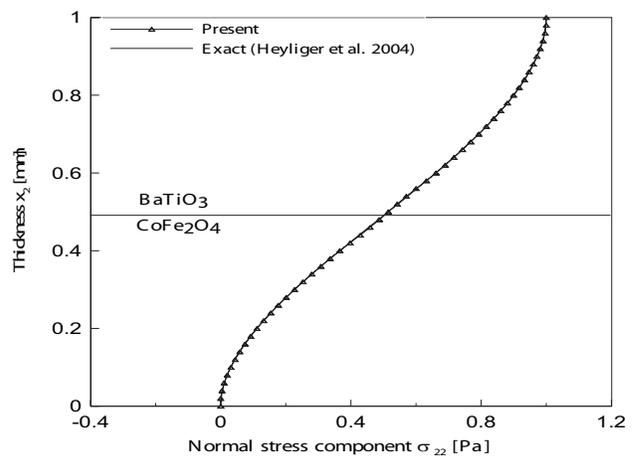
**Figure 8** : Through thickness behavior of  $\sigma_{22}$  stress component.
