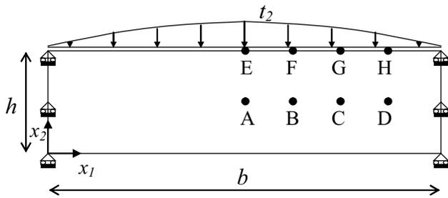
Figure 2 : Magneto-electro-elastic beam scheme.
