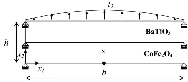
Figure 4 : Magneto-electro-elastic laminate scheme.
