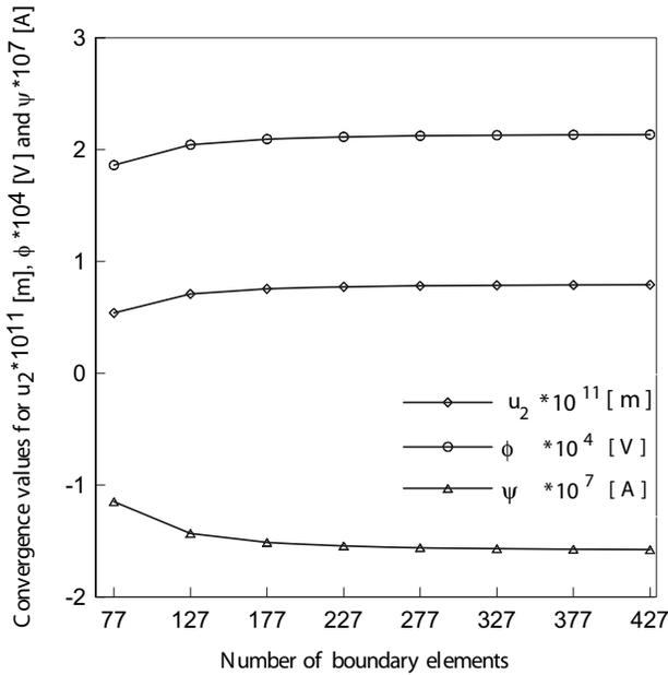
**Figure 5** : Convergence analysis for the point  $X \equiv (b/2, 0)$  of the magneto electro elastic simply supported laminate.
