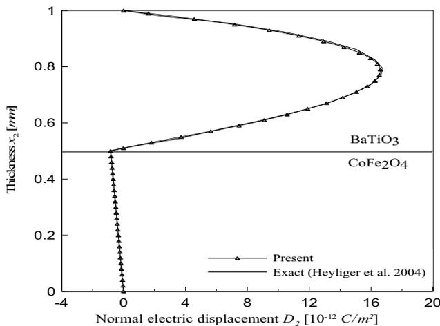
**Figure 11 :** Through thickness distribution of the normal electric displacement component  $D_2$ .
