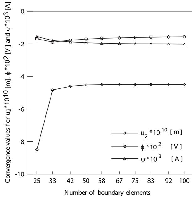
Figure 3 : Convergence analysis for the point E of the magneto-electro-elastic clamped beam.
