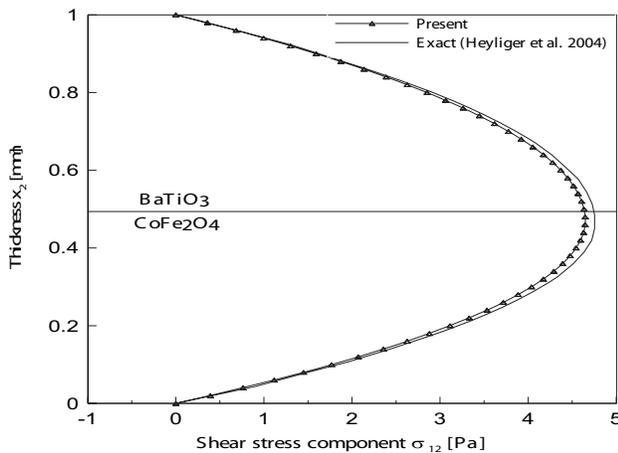
**Figure 9 :** Through thickness distribution of the transverse shear stress  $\sigma_{12}$ .
