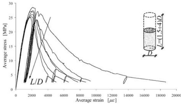
Figure 1 : Size effect for the  $\bar{\sigma} - \bar{\epsilon}$  diagrams
