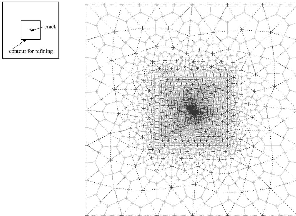
**Figure 21 :** Local mesh generation for a cracked plate with refining on an internal contour and on the crack, when the interaction between  $n$
