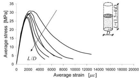
**Figure 26 :** Numerically evaluated size-effect on average stress-average strain diagrams (see Fig. 1)
