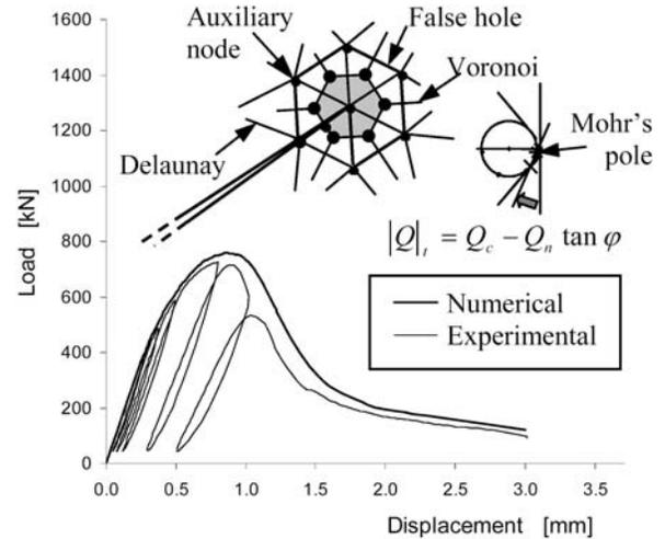
**Figure 25 :** Comparison between numerical and experimental results for compressed concrete specimens
