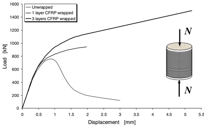
**Figure 29** : Numerical load-displacement curves for unwrapped and CFRP wrapped specimens
