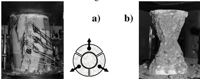
Figure 3 : Concrete specimen at the end of the test, with scheme of splitting on the middle cross-section (a), and concrete specimen at the end of the test, after removal of the outer part (b)
