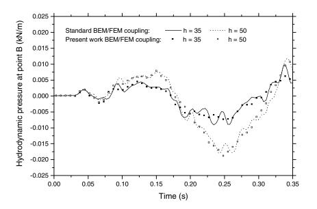
Figure 7 : Hydrodynamic pressure at point B: influence of the water level.
