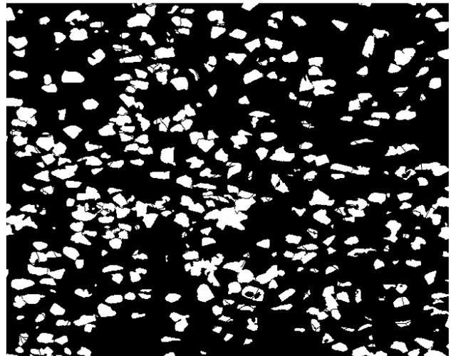
**Figure 1** : Binary image of the Al/SiC composite.
